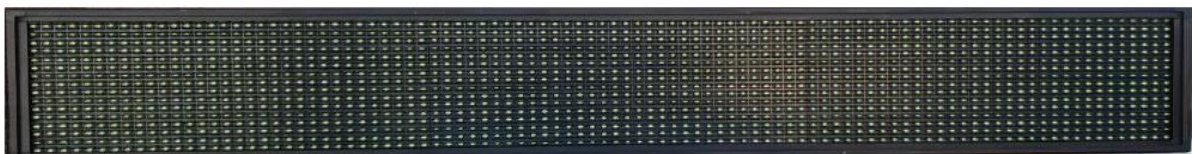
Figure 1: LED display 96x16 unlit diode
